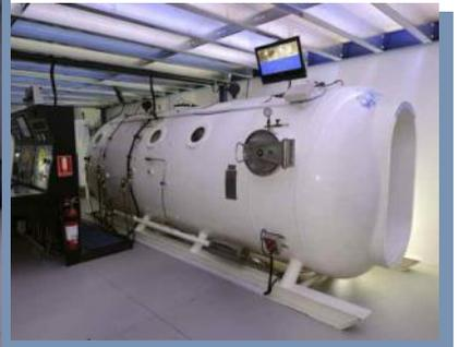
The PDS Twin lock Hyperbaric chamber with walk-in entry into the Main Lock features some of the latest technology. Fully equipped with Oxygen supply, lighting, communications, video surveillance and sound system, this Hyperbaric unit is located at our Unit 10 Facility at our Banksmeadow address.
