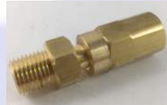
P/N: PDS-HE205 Hose end to suit 8mm Air hose 1/4" Male NPT thread
