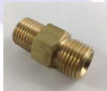
P/N: PDS-NIP303 9/16" UNF Male thread with cone to Male 1/4" BSPP
